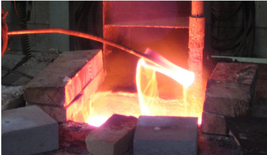
Figure 9-11: Open air NaCl-KCl Salt bath at 900oC for metal heat treating. (Picture taken at Metallurgical Solutions, Inc in RI)
