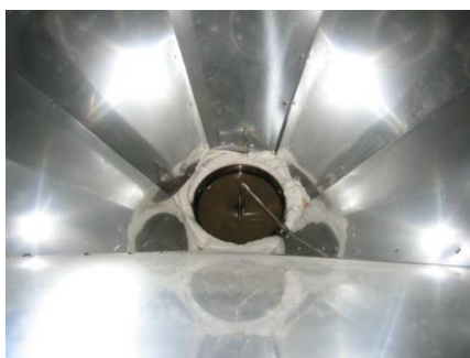
a: Volumetric receiver inside solar simulator output aperture.
