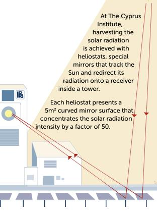
Our field of heliostats at the PROTEAS facility on the southern coast of the island yields an intensity of 2,500 suns, reaching temperatures in excess of 1,000°C. The sunlight is converted into heat, which is stored for later use in a tank filled with high temperature molten salt. This means the solar energy can be used anytime, on cloudy days and at night. The stored energy is used for the cogeneration of electricity and desalinated sea water.
